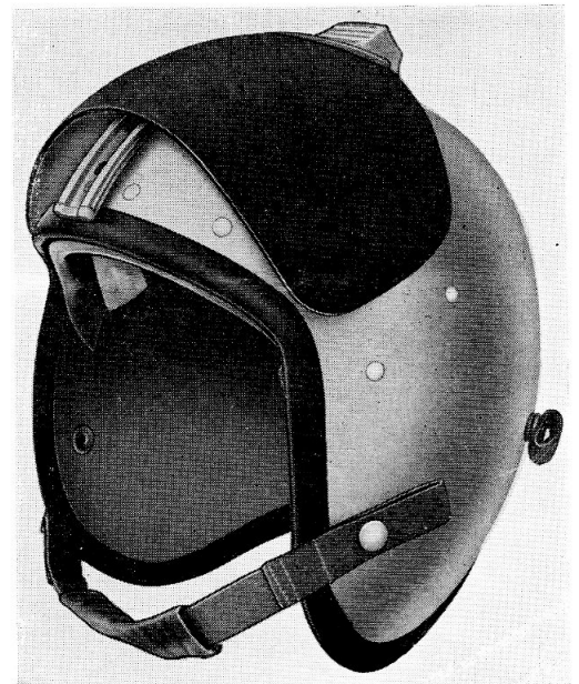
Fig. 3. Mk. 2C visor fitted to a Mk. 1A helmet : up position
