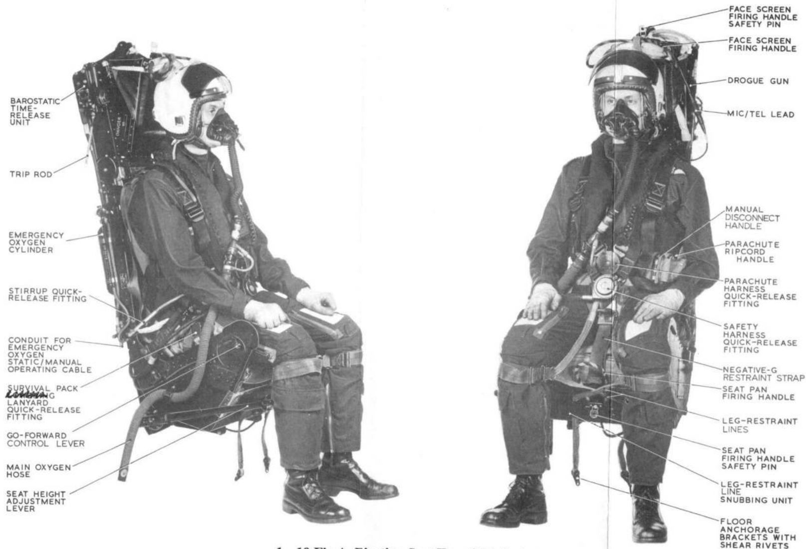
1-10 Fig 4 Ejection Seat Type 2CA Series (Terminology Amended)
