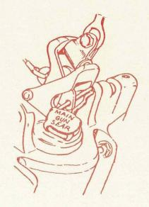
SAFETY PIN THROUGH BREECH TIME DELAY FIRING UNIT SEAR (MK T5)
