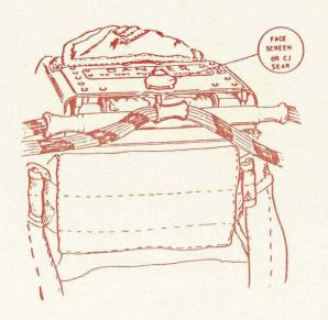
SAFETY PIN SECURING EJECTION SEAT FACE SCREEN FIRING HANDLE.
