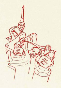
MAIN GUN SEAR SAFETY PIN THROUGH THE BREECH TIME DELAY UNIT AND FACE SCREEN SAFETY PIN THROUGH CANOPY JETTISON UNIT SEAR (MKS 3 AND 6 AIRCRAFT).
