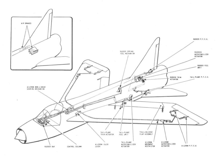
FIG.1. GENERAL ARRANGEMENT OF FLYING CONTROLS
