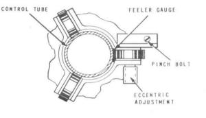
A TOLERANCE OF +0.005 IN TO 0.010 IN. TO BE MAINTAINED FOR ALL CONTROL ROD RUNS THROUGH ROLLER GUIDES 1-8352-1
