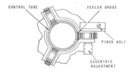
A TOLERANCE OF  $^+$  0.005 IN. TO 0.010 IN. TO BE MAINTAINED FOR ALL CONTROL ROD RUNS THROUGH ROLLER GUIDES
