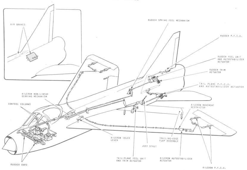
FIG. 1. GENERAL ARRANGEMENT OF FLYING CONTROLS
