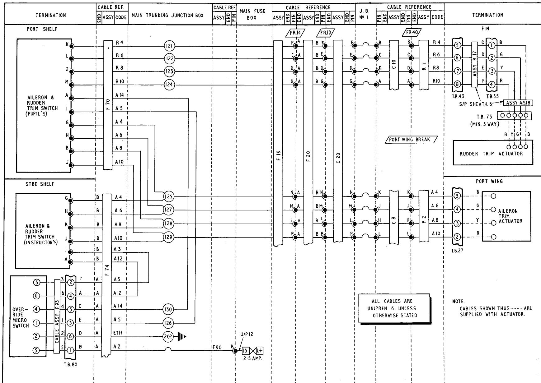
Fig.2. Rudder and aileron trim control (routeing)
