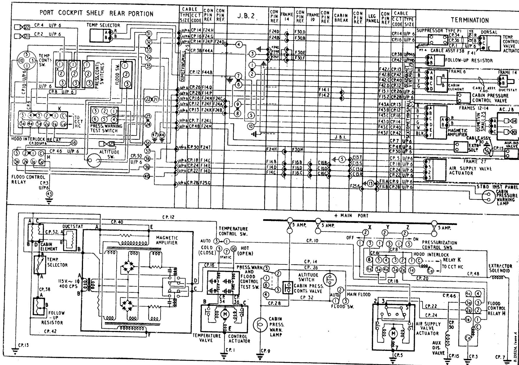
Fig.1. Cabin pressurization and temperature control (routing and theoretical)
