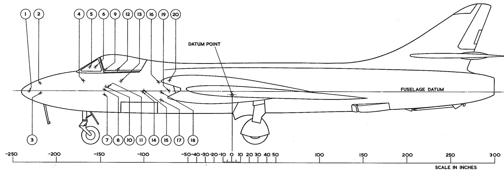
FIG. I. LOADING AND C.G. DIAGRAM
