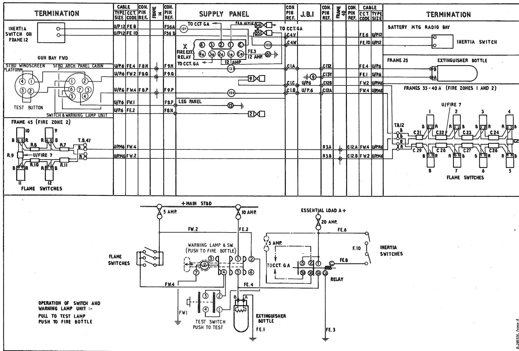
Fig. 1. Fire warning and extinguisher (routeing and theoretical)
