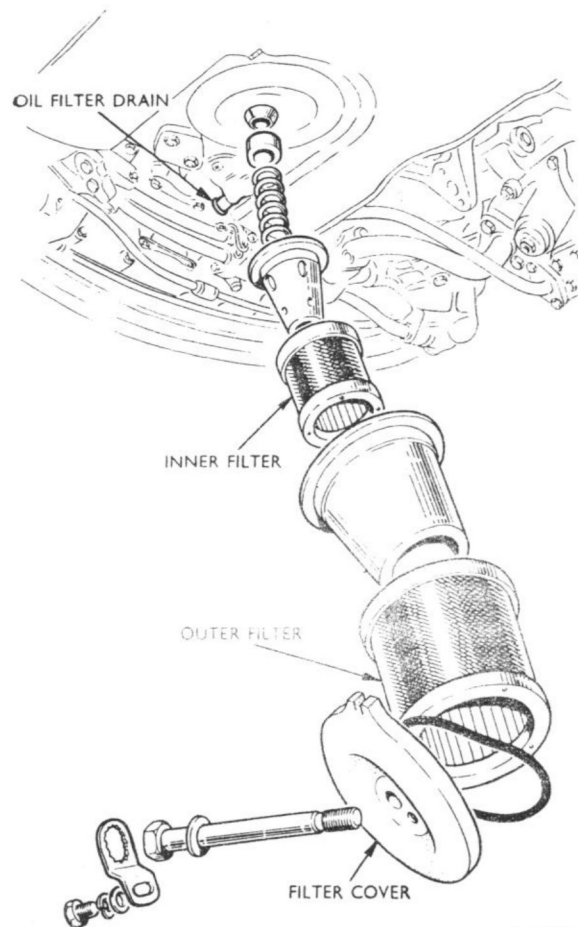
Removing the pressure oil filter Fig.2
