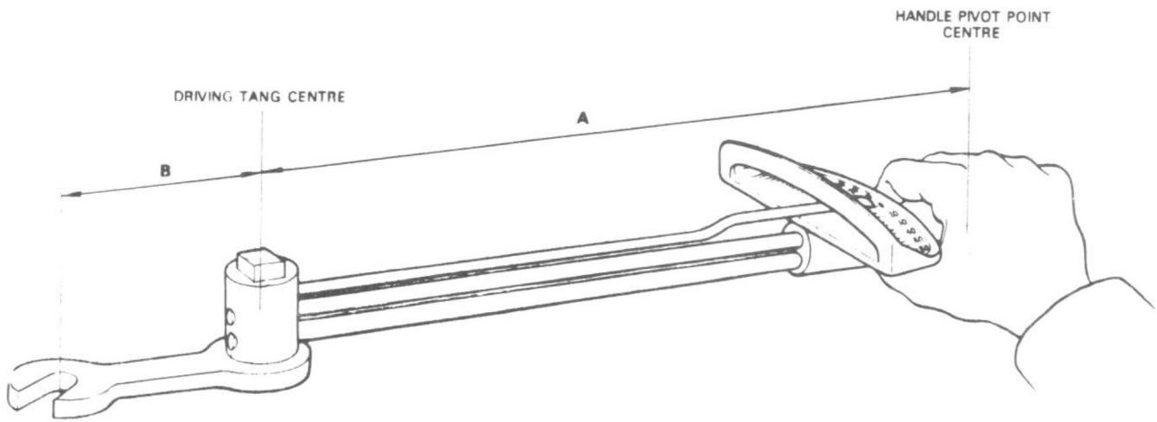
Correct method of using extension spanner with torque wrench
