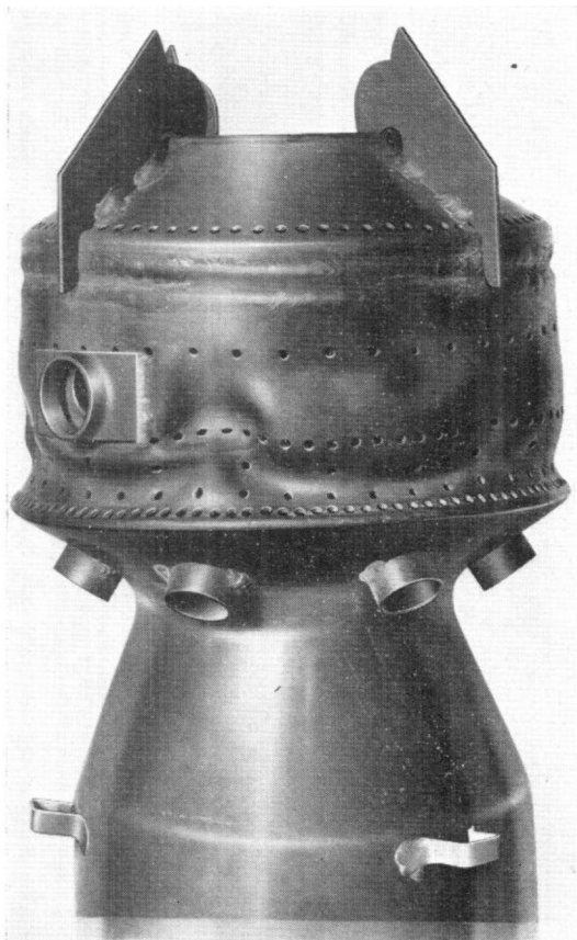
Fig. 5. Unacceptable damage to the flame tube primary zone
