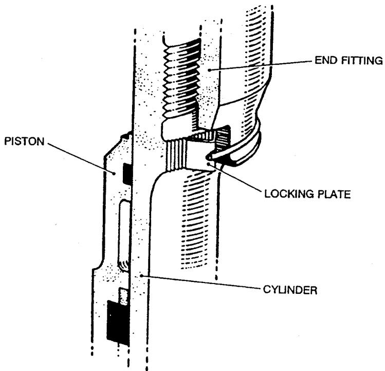
Fig 2 Right-angled locking plate in position
