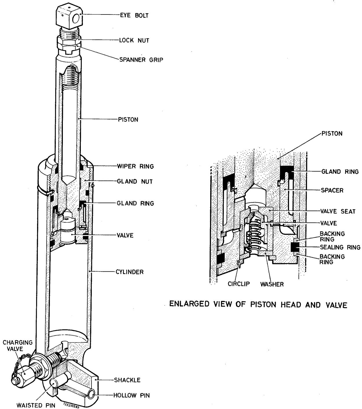
ENLARGED VIEW OF PISTON HEAD AND VALVE
