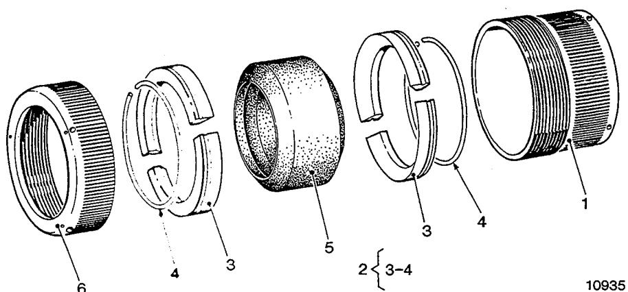
Fig 12 Pipe Connector
