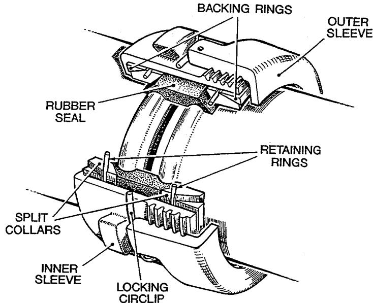
Fig 3 Pipe connector, FRS 325
