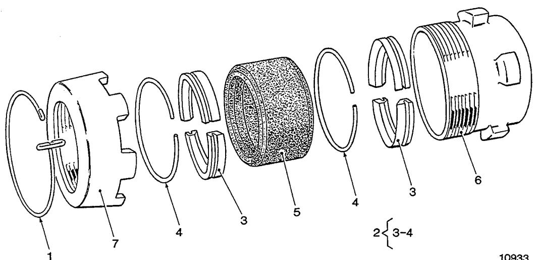
Fig 10 Pipe Connector
