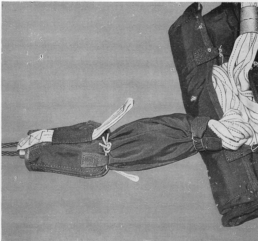
Fig. 15. Gaiter secured over connection: breaking tie loop passed through gaiter tunnels
