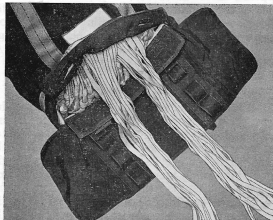
Fig. 8. First section of rigging lines stowed on top of canopy
