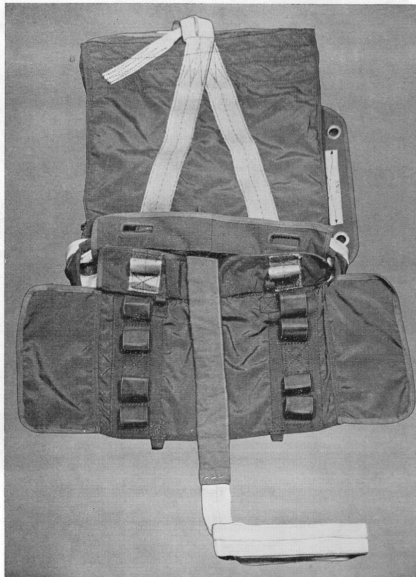
Fig. 1. Pack: outside: flaps opened to show apex strop sleeve
