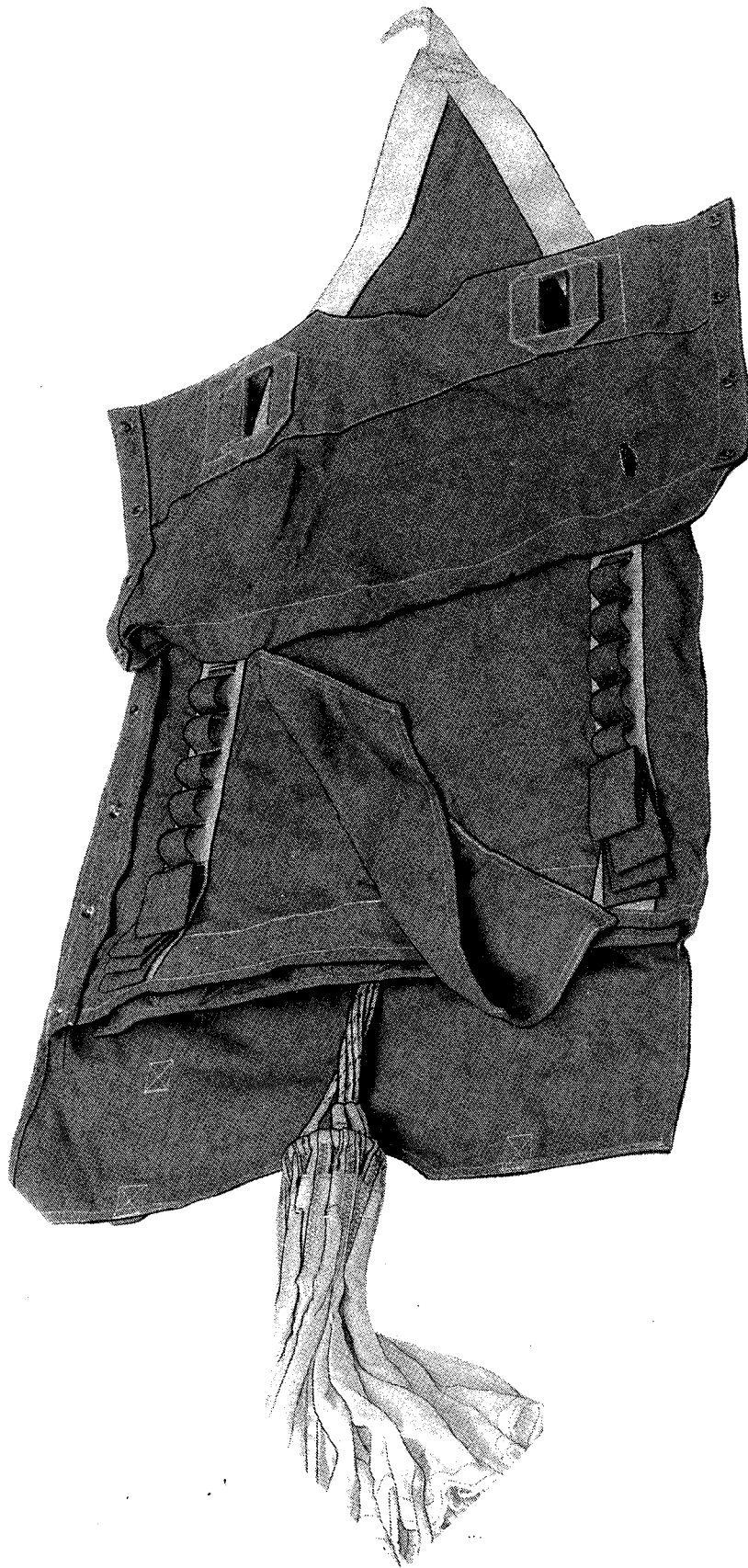
Fig 2 Pack showing strop and cable stowage
