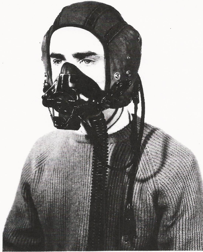
Fig.1 Type G helmet worn with oxygen mask
