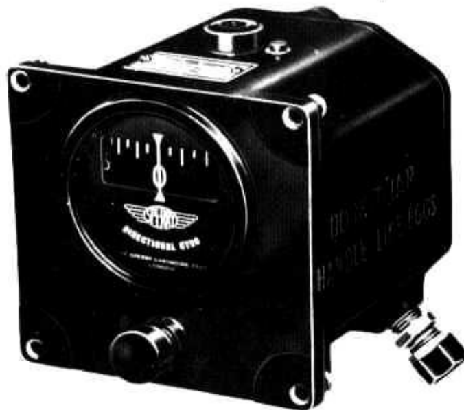
Fig. 1. Directional gyro, Sperry, Type D.L.2
