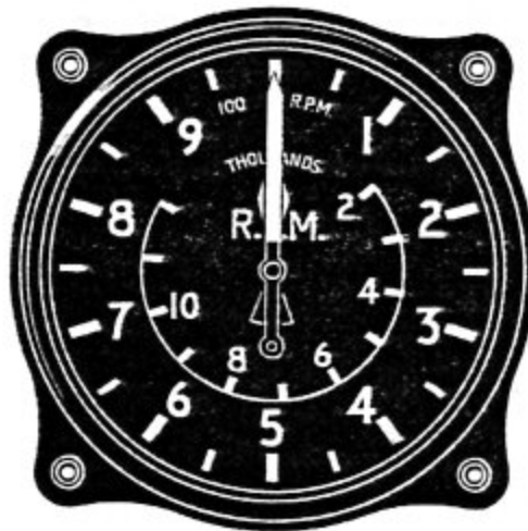
Fig.1 Tachometer indicator - dial presentation
