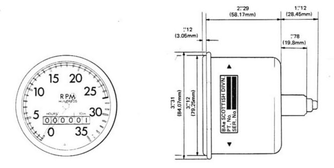
Fig.1 Tachometer indicator, Type RT7
