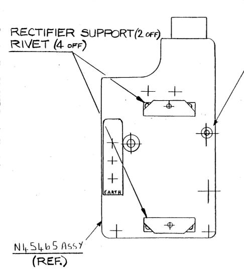
REMOVE AND DISCARD SCREW NL519L COUNTERSINK EXISTING HOLE TO 0.218 O.228 DIA. × 90° FROM THIS SIDE.
