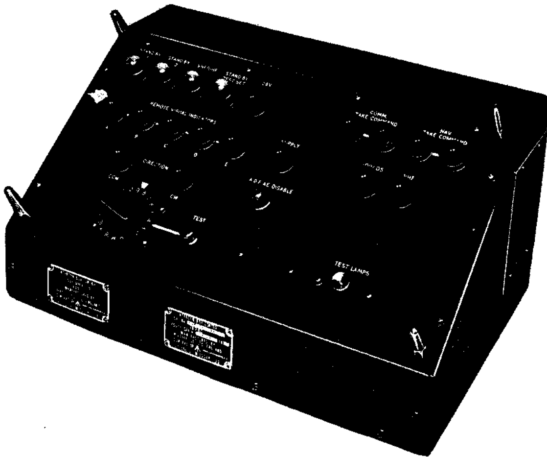
Fig. 13. Control, interconnecting box, test set 6625-99-194-5272
