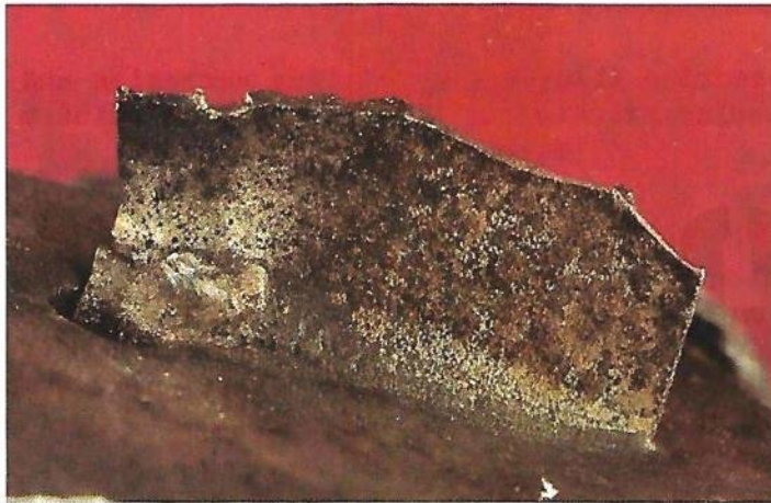
Fig 14 Pitting corrosion on a Gnome engine compressor stator blade
