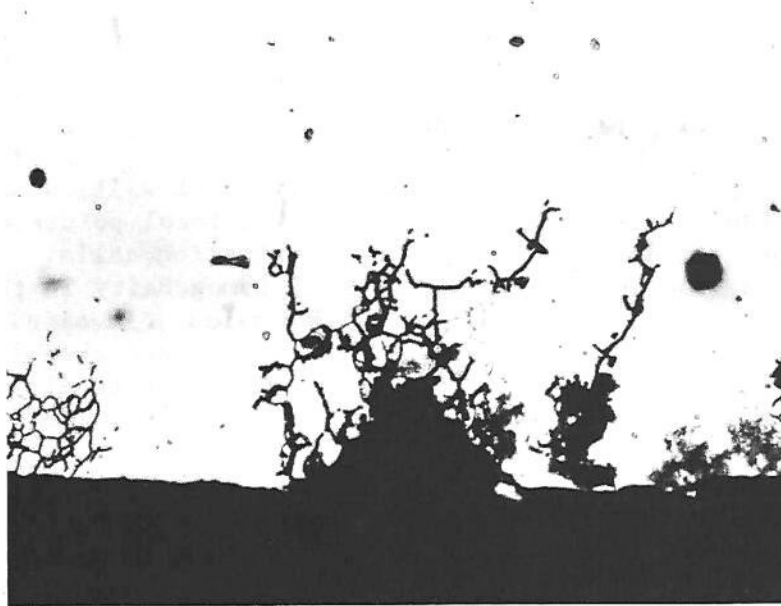
Fig 16 Microsection illustrating pitting corrosion and associated intergranular cracking in the surface of aluminium alloy (magnified 500 times)
