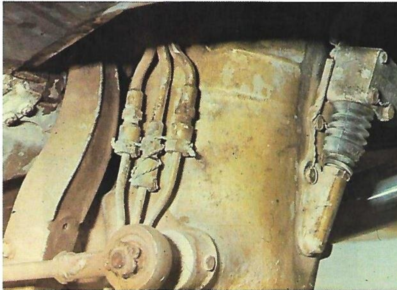
Fig 3 Sand adhering to undercarriage components
