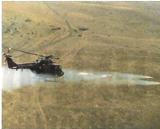
Fig 7 Lynx helicopter weapon firing, illustrating exhaust deposition (Westland Helicopters)
