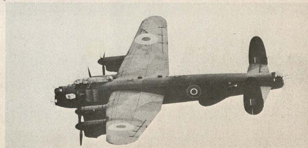
LOW LEVEL over the crowd at Filton, showing upper-surface markings, including 'walk lines' on the wings. The two protrusions on the fuselage behind the astro-dome are housings for French radar aerials, and have now been replaced with the more standard 'whip' aerials. (E. Ashman)
