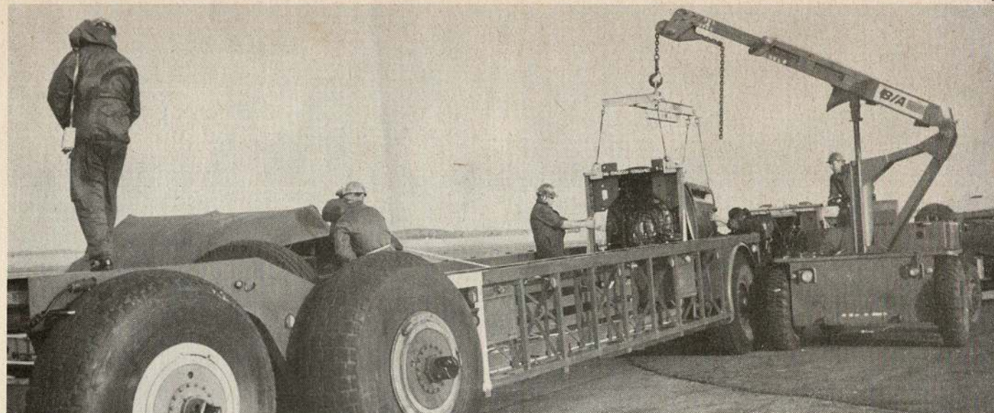
Above: TIGHT FIT. With only an inch clearance each side, an engine is edged aboard a "Queen Mary" trailer, beside which stand the Lanc's mainwheels. (Brian Goulding)
