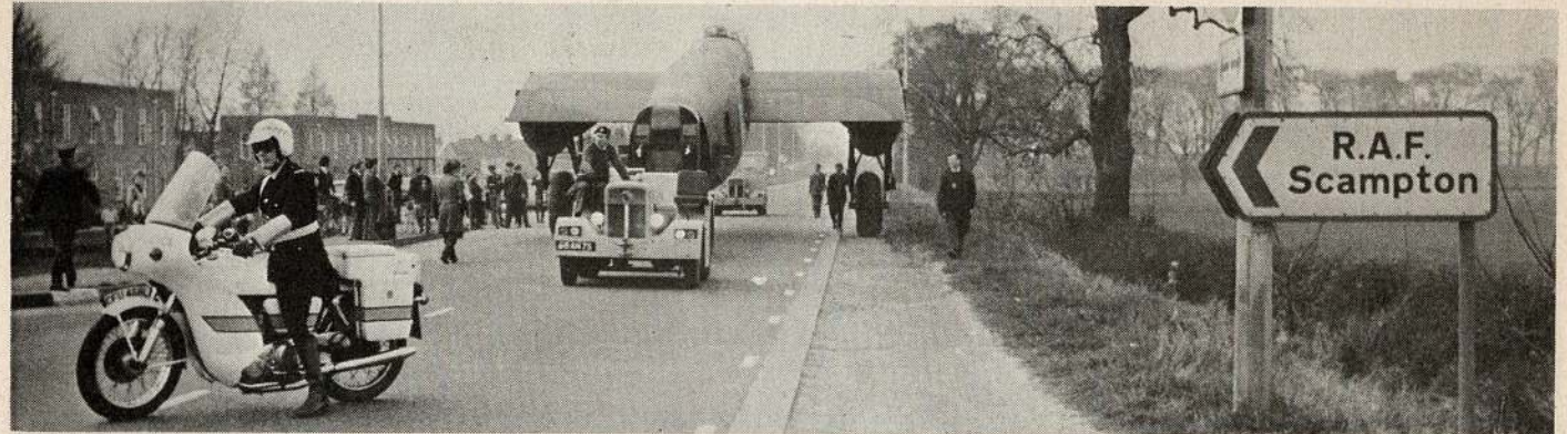
HOLD UP on the A15 as NX611 is towed towards the main gate ready for final positioning, wings and tail removed for transit. (Lincolnshire Echo)
