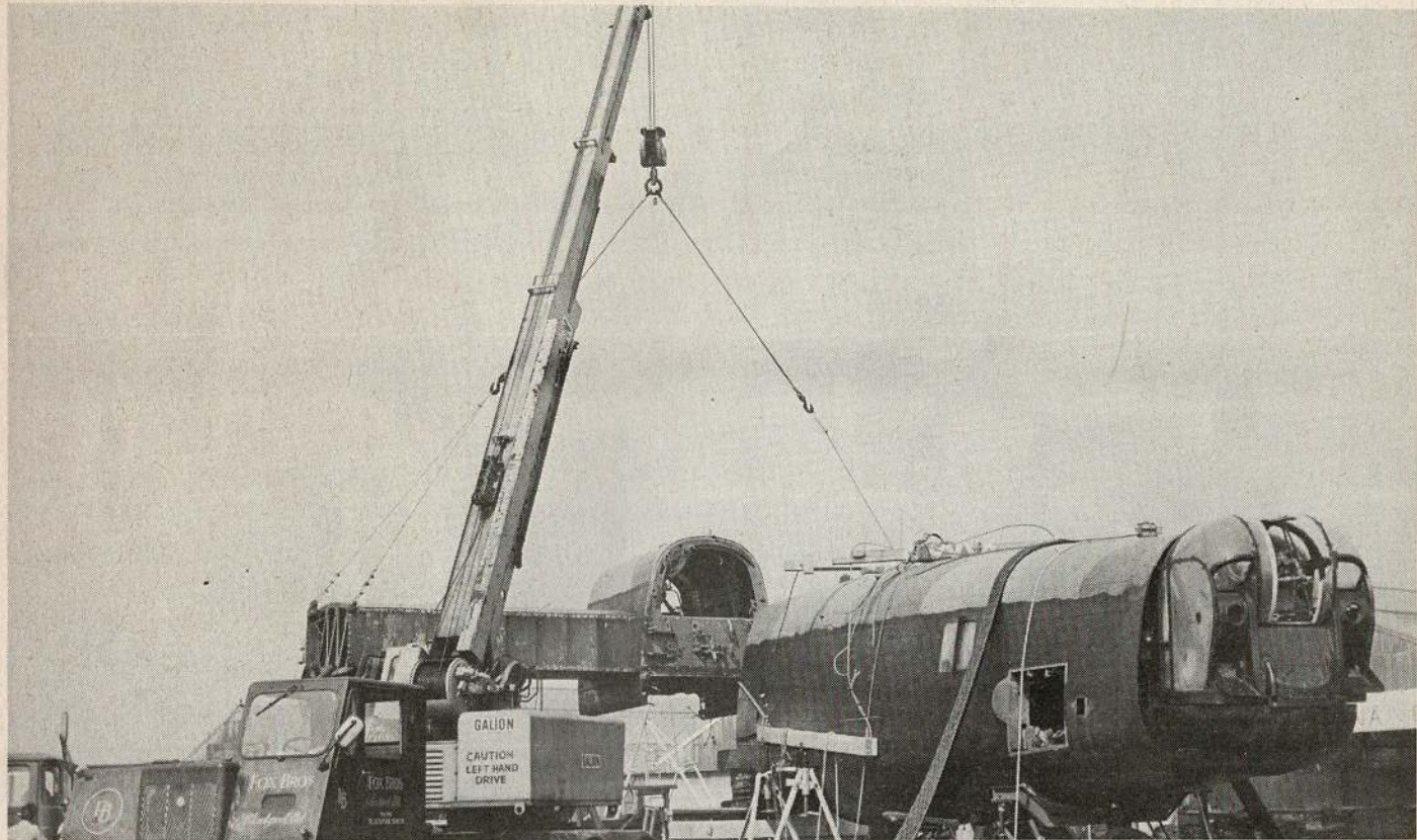
FINAL PARTING as centre section and rear fuselage are separated. The centre section itself constituted one complete trailer load, the biggest and most awkward one of all, requiring police escort through built-up areas (RAF Scampton Photographic Section)
