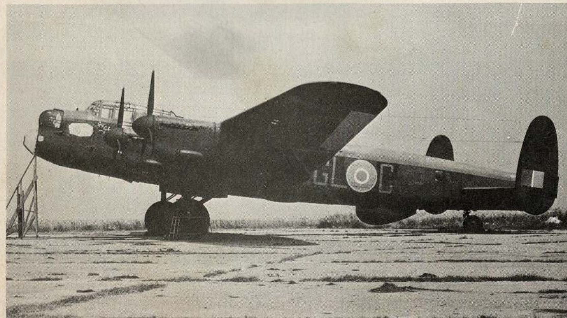
NEW HOME, NEW MARKINGS (below), August 1969. The codes GL-C were applied following a visit by Gp Capt G. Leonard Cheshire, VC DSO DFC. Shortly before leaving Biggin Hill the ailerons had been removed and sent to Hawker Siddeley's Woodford factory for refurbishing, and the new fabric stands out clearly on both photo's. (Lewis G. Pain)
