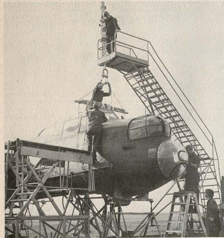
Above : SEPARATION of port wing spars. Removal of one wing tip alone involved the unscrewing of 96 nuts. Some corrosion is evident at the facing joints. (RAF Scampton Photographic Section)
