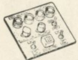
ENGINE START CONTROL PANEL (PORT CONSOLE)
