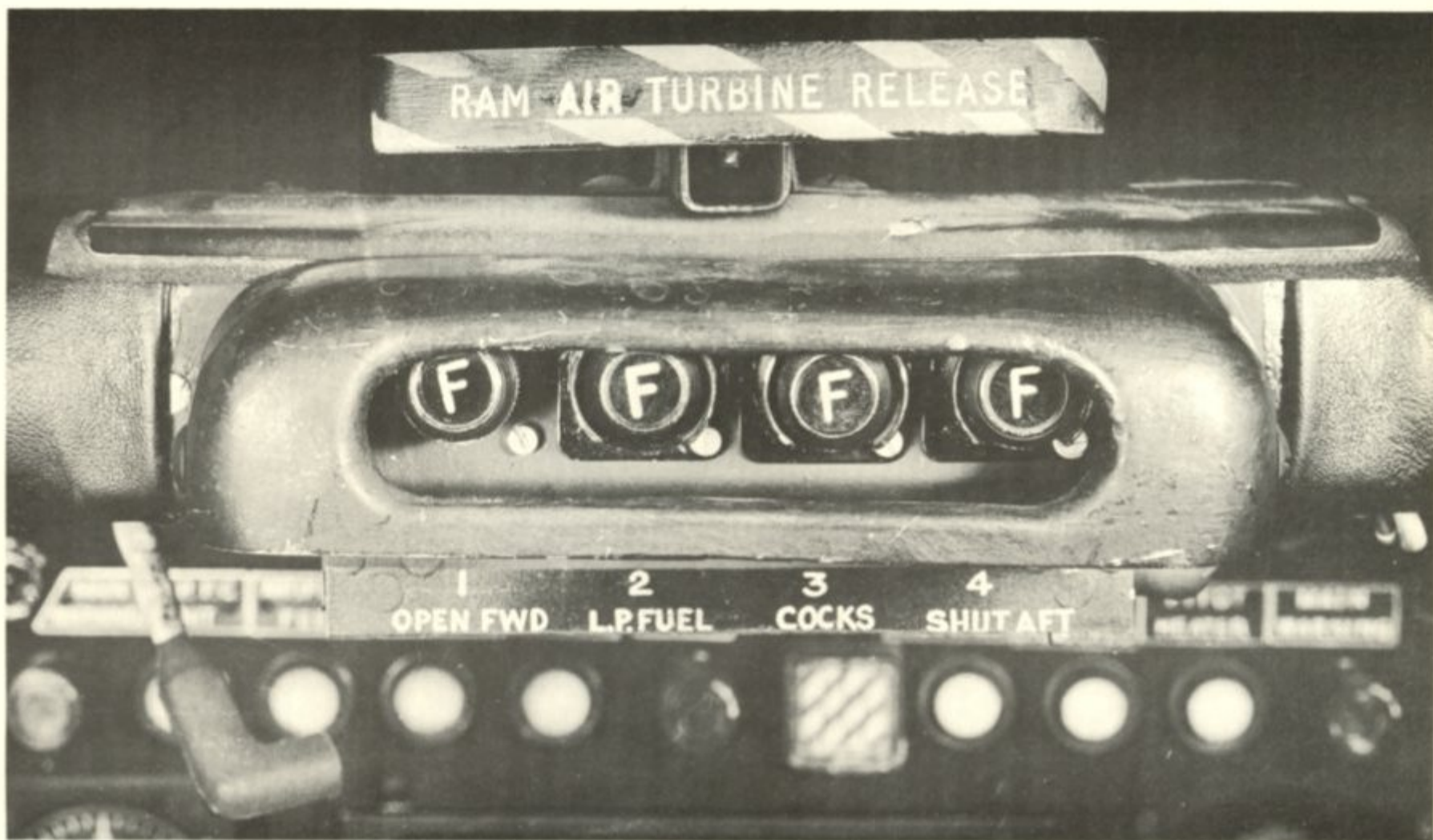
Figure 2, Fire Warning Switches.
