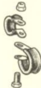
PIPE CLIP DETAIL AT L
