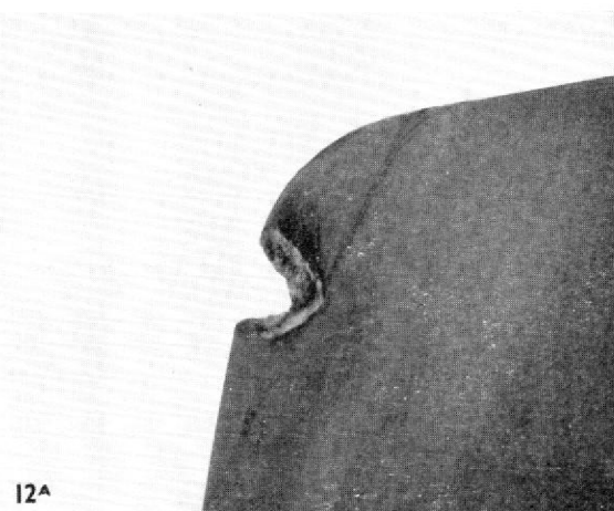
Fig. 51. An enlarged view of the damage shown in Fig. 50 (magnification \times 4 ) which enables the ragged nature of the indentation to be seen clearly.
