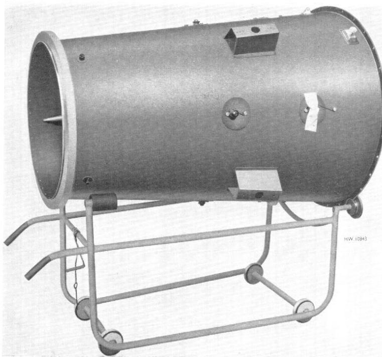
Fig. 1. Exhaust cone assembly mounted on stand T.75700. The large ring, which is attached by wire to the rear end of the outer cone, will provide support at this point during dismantling and re-assembling.
