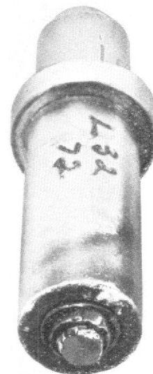
Fig. 6 (2 left). R.I pellet satisfactory but centre electrode burnt—reject.
