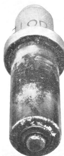
Fig. 10 (14 left). Slight burning of centre electrode and slight flaking of R.I pellet—serviceable.
