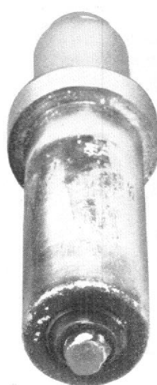
Fig. 4 (6 left). Centre electrode burnt and R.I pellet flaking—reject.
