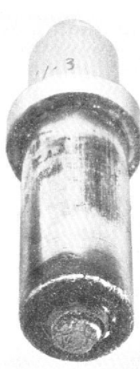
Fig. 10 (14 left). Slight burning of centre electrode and slight flaking of R.I pellet—serviceable.
