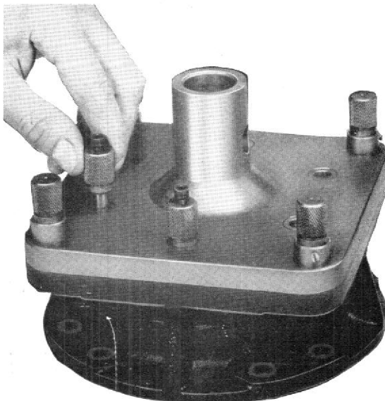
Fig. 111. Checking alignment of clearance holes.
