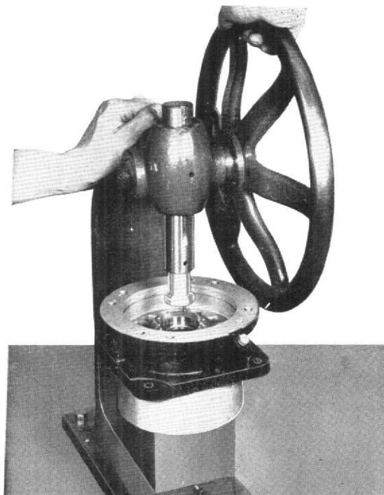
Fig. 52. Using rack press NT.864, base NT.4008B and punch NT.4010 press out the oil seal. Note: Once removed, the oil seal cannot be refitted and must be renewed.
