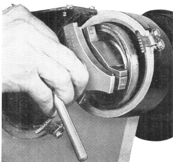
Fig. 30. Using tool NT.4007, remove the "Clupet" seals. Make sure that the jaws of the tool are well behind the seal. It may be necessary to clean out the carbon deposited behind the seal to allow the jaws to fully expand.
