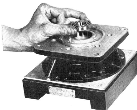
Fig. 50. Remove front bearing as shown. The bearing spacer located between the front and rear bearings can now be withdrawn. (For this operation the housing is removed from securing tool NT.4011, turned over and placed on bench block NT.4012.) Remove the three screws and tab washers securing the rear bearing clamp plate and remove plate. Remove the rear bearing, tapping the casting if necessary to ease it. Note: It is advisable to wrap these bearings to protect them.
