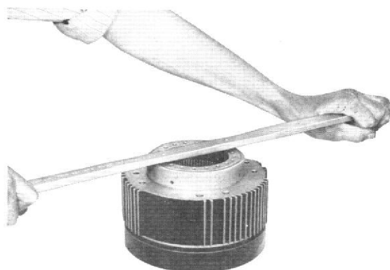
Fig. 45. Using bench block NT.4005 and clutch adjusting bar NT.4006 remove clutch adjusting nut and clutch springs. Caution: Tape the thread of the clutch nut to protect it from damage.
