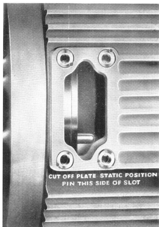
Fig. 19. Inspection of cut-off plate.
