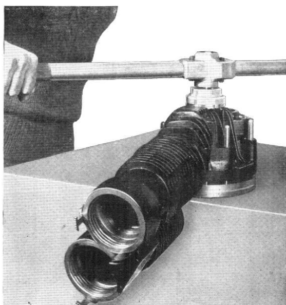
Fig. 33. Remove centre plug. Fit tool NT.4107 in position by means of a \frac{1}{8} in. (AF) Allen Key, and, using spanner NT.5171 remove the cap nut (it may be necessary to warm the casting).
