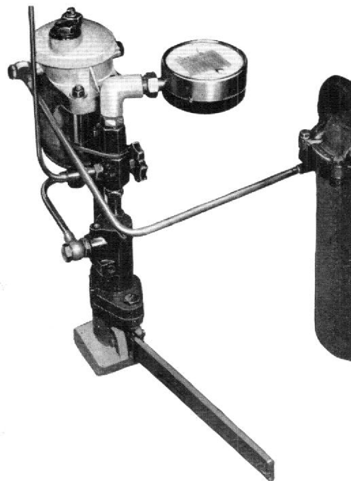
Fig. 70. Hydraulic test pump.
