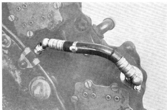
Fig. 3. Failure of flexible pipe caused by using the incorrect method of fitting.
