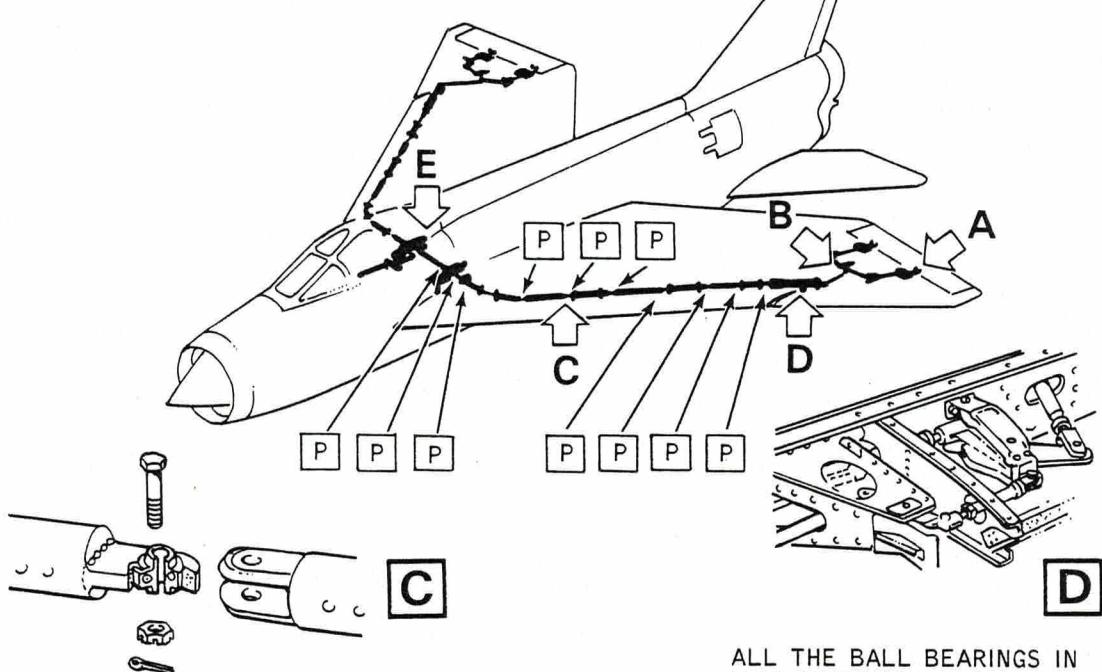
TYPICAL ROD-TO-ROD CONNECTION, PRE-PACKED
