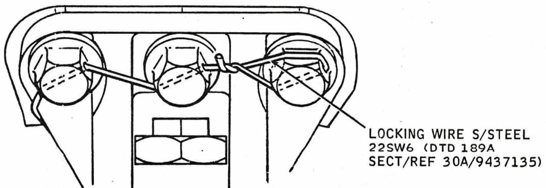
WIRE LOCKING AND SEALING OF BOLTS
