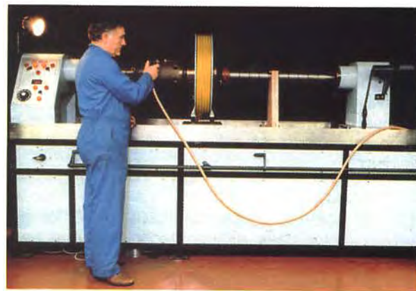
Fig. 25-3 Magnetic crack testing.
