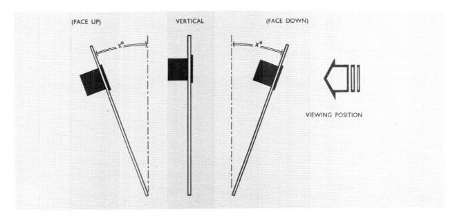
Instruments may also be calibrated for use in the horizontal plane.
