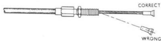
Fig. 8 Alignment of conduit and cable
