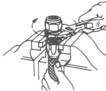
Fig.15 Tightening the nipple assembly
