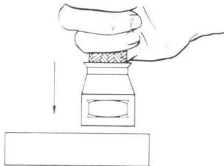
Fig.3 Loosening the 'SuperGem' socket
