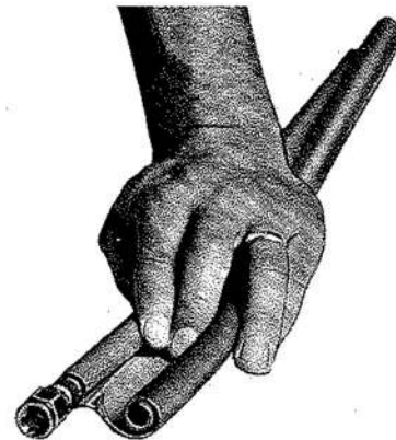
Fig 24 Wrap sleeve onto hose
