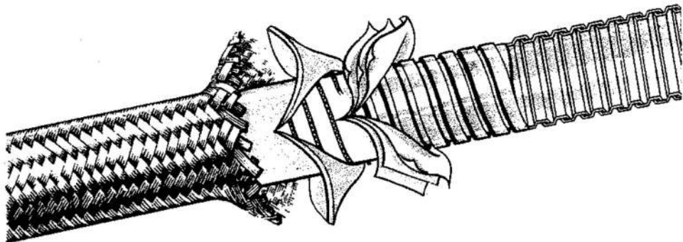
Fig 1 Avioflexus hose construction
