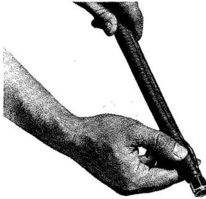
Fig. 26 Work out excess adhesive
