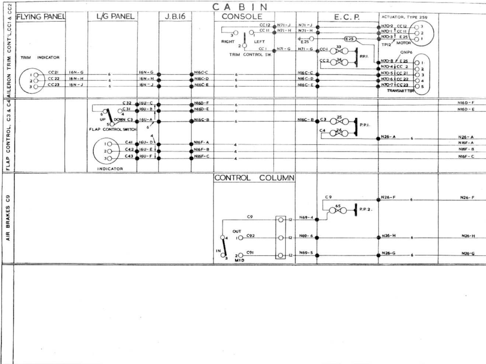
FIG. 8. AILERON TRIM CONTROL - AIR BRAKES - FLAP CONTROL
