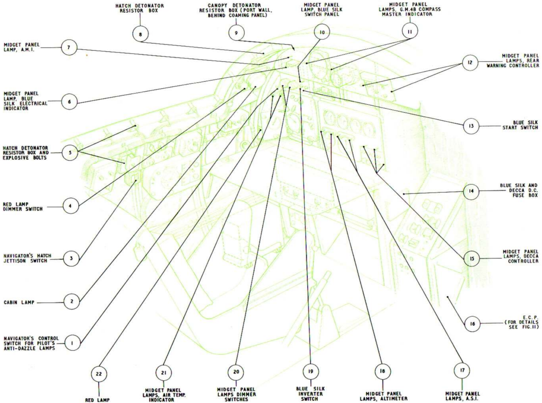
Fig. 5. Electrical installation - navigator's station (B (I) Mk.6 aircraft)
