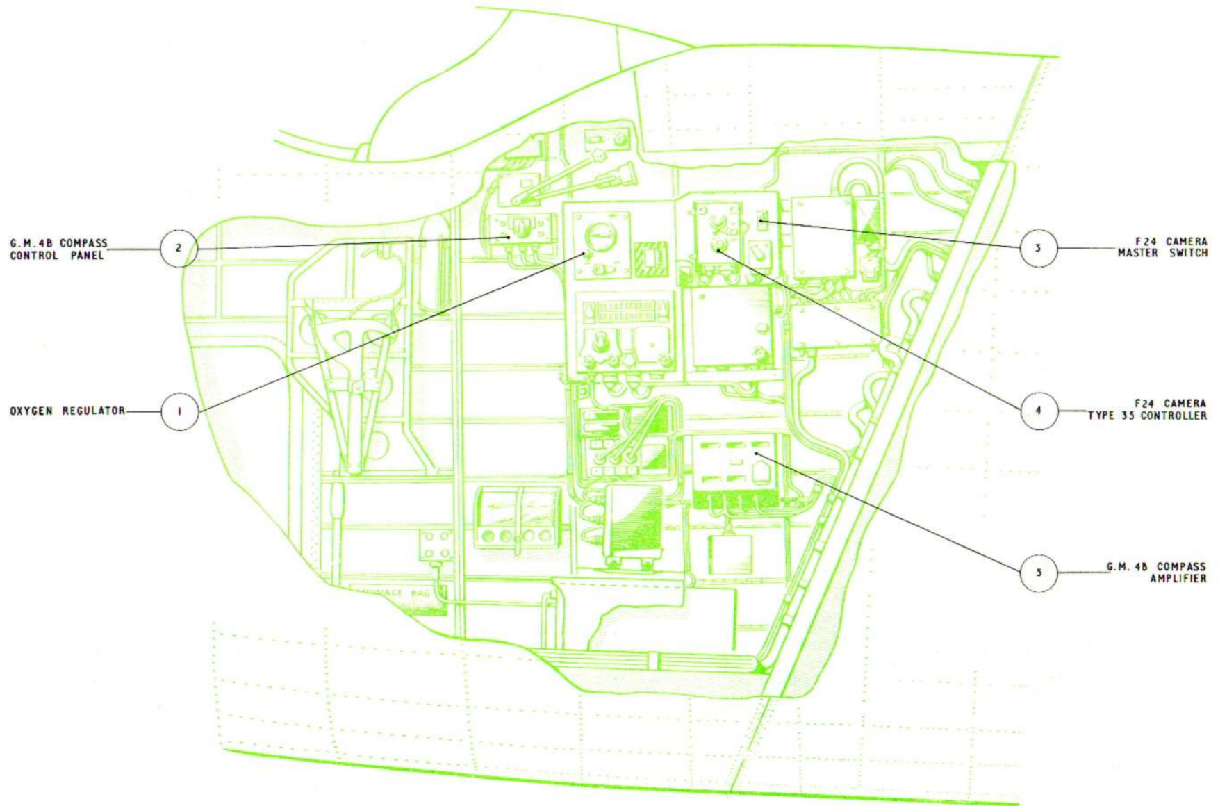
Fig. 8. Instrument installation – air bomber's rear station (B Mk.6 aircraft)
