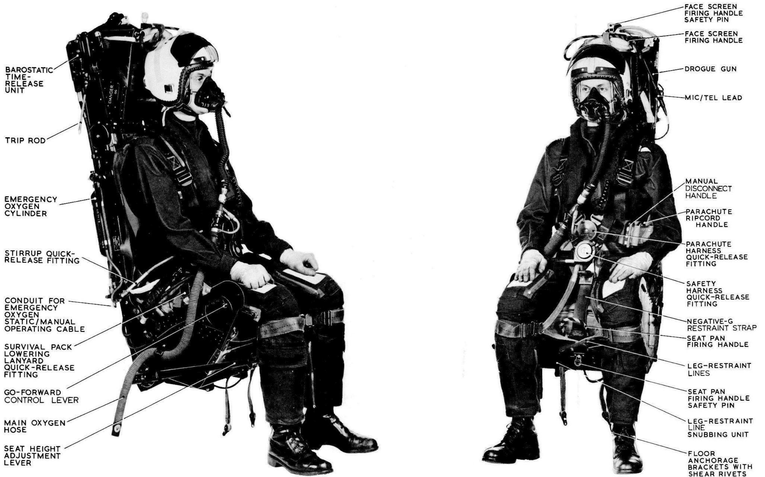
1 - 10 Fig 1 Ejection Seat Type 2CA Series (Terminology Updated)
