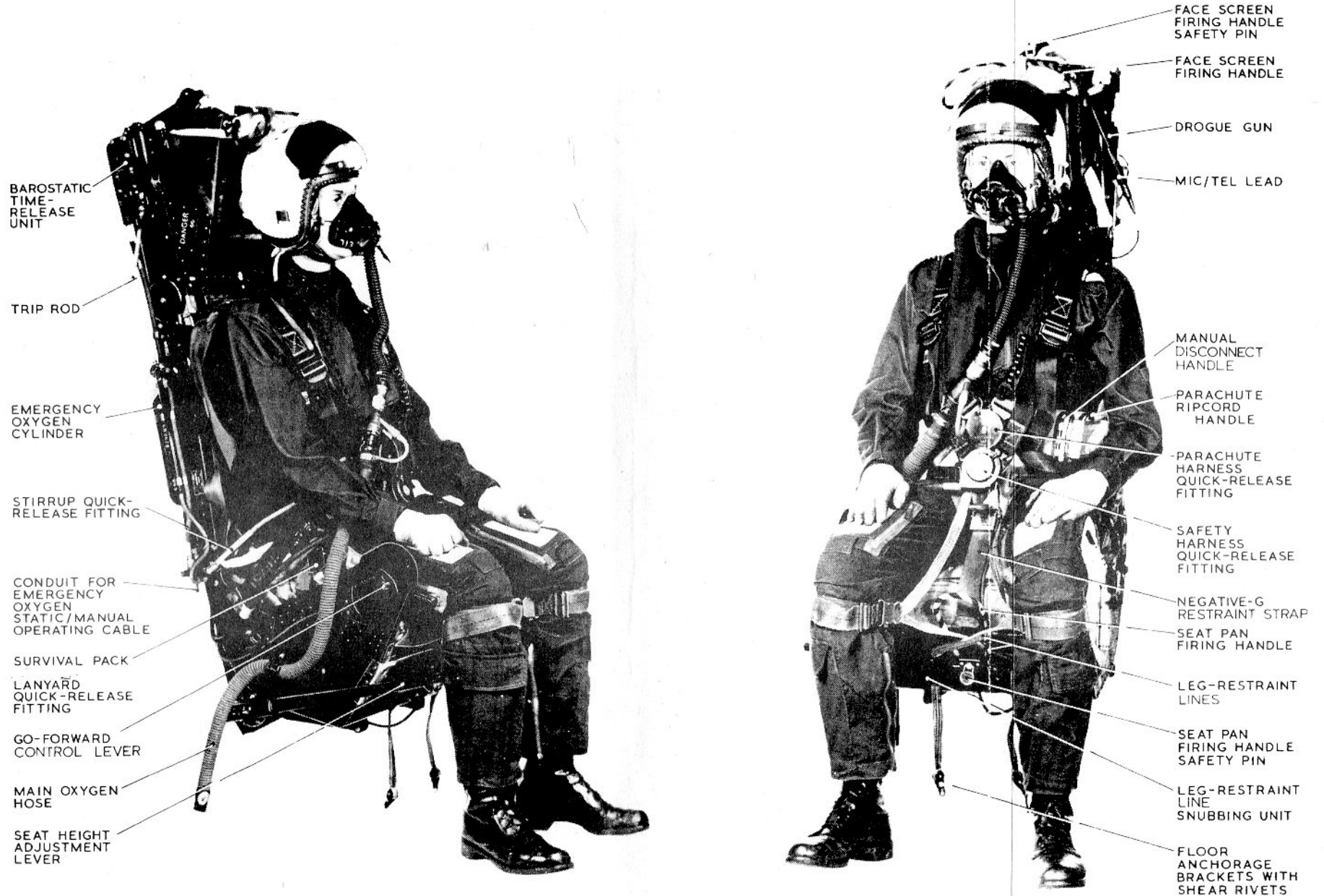
Fig 1 – Ejection Seat Type 2CA Series ◀ (Terminology Updated) ▶
