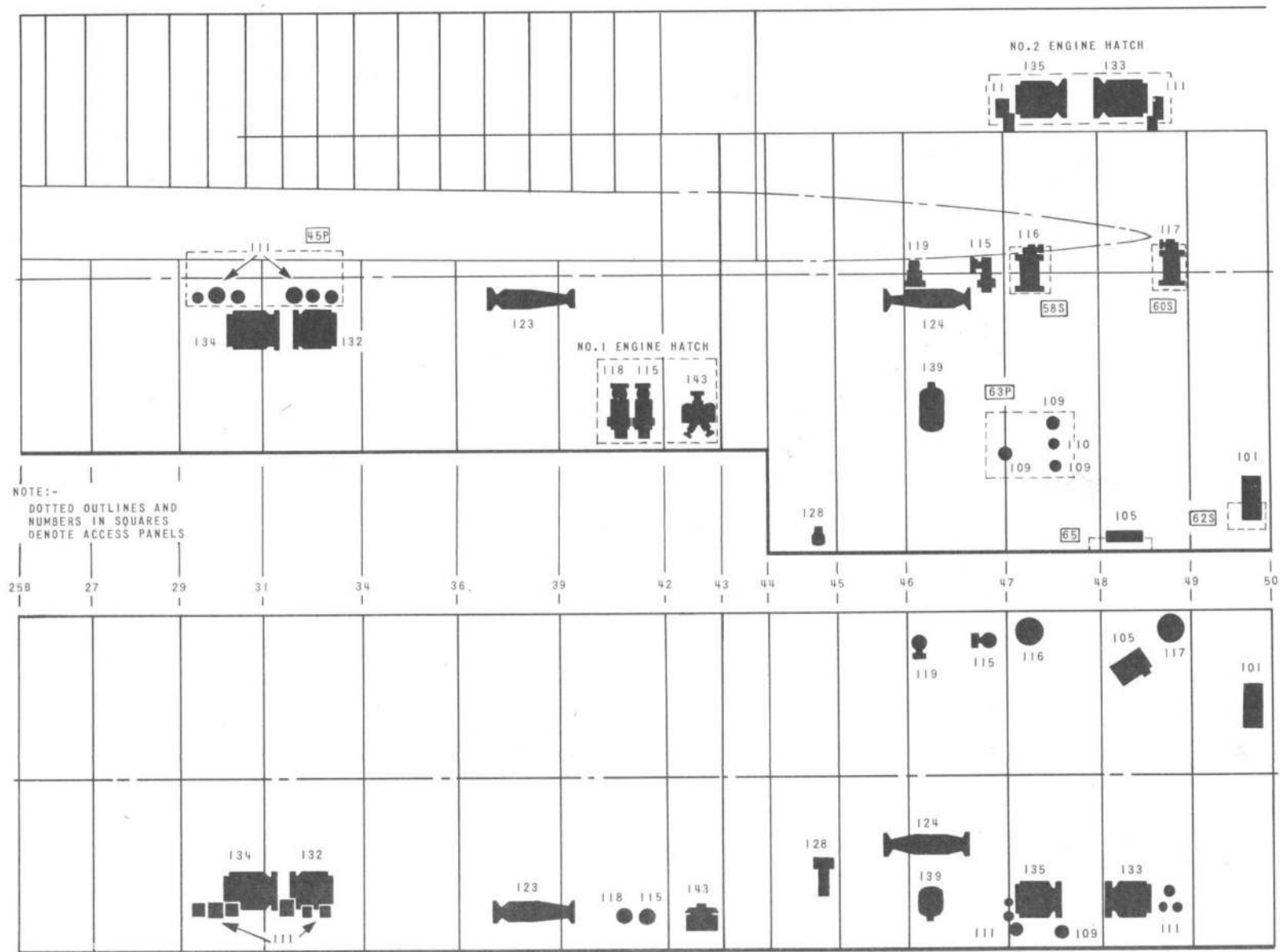
FIG.9. LOCATION OF MAJOR COMPONENTS - FRAMES 25B-50
