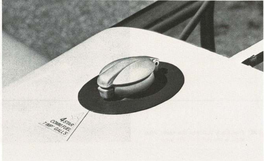
Fig 33 Tank cap of the 7 gallon fuel tank
