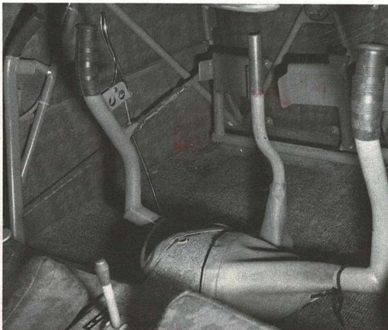
Fig 29 The crew sit side by side and both have a full set of flying controls. In this picture you can see the two control columns (the one on the left has the brake operating lever) and the two spoiler operating levers. (The short lever between the seats is the elevator trimming control). Fig 30 shows the rudder pedals more fully.
