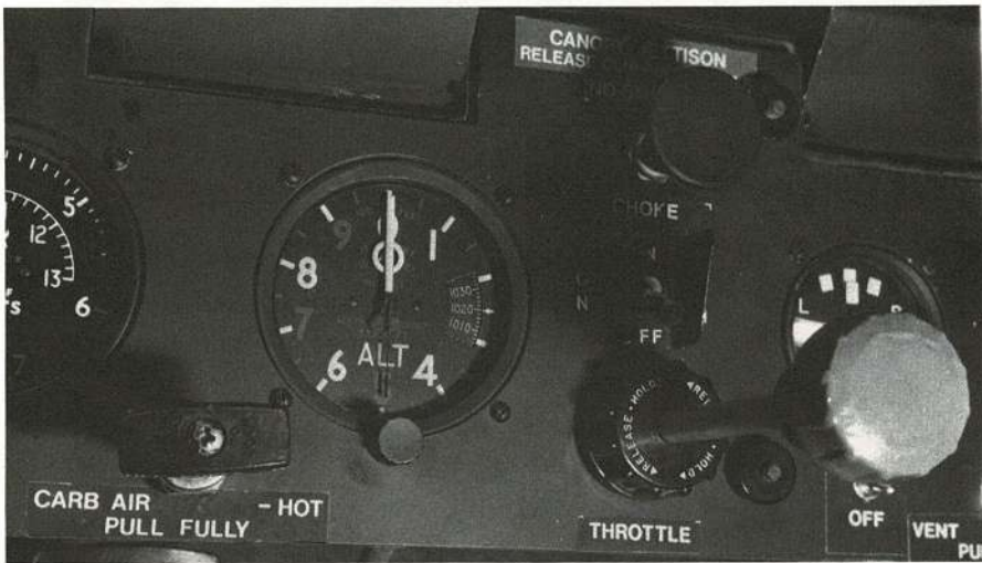
Fig 32 The throttle is the long knob in the centre of the panel. "IN" to "OPEN".
