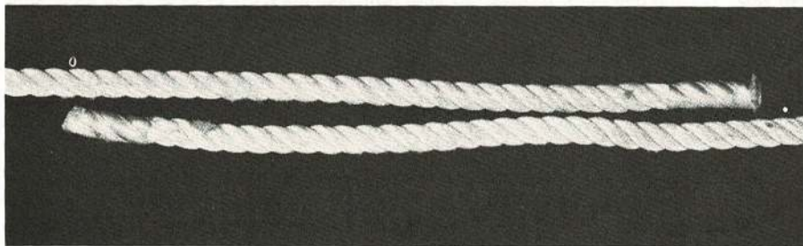
Fig 18A Lay the two running ends together . . .
