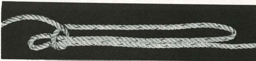
Fig 33B Cast a clove hitch over one end ....
