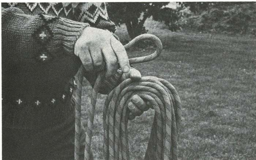
Fig 9F Then form a loop in the final piece of rope and lay it along the coil (as for a whipping).
