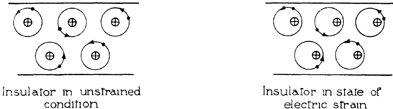
FIG. 3, CHAP. I.—Displacement current.
