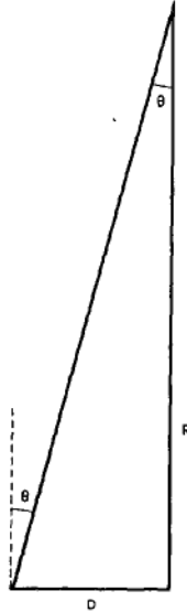
Fig.A: Principle of optical range-finder
