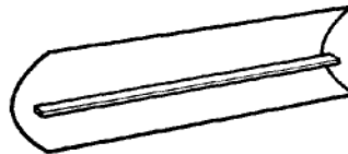
Fig.840.- Waveguide array feeding parabolic cylinder.
