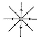
Fig. 744. - Electric field around charge moving with uniform speed.
