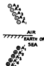
Fig.815.- Image of array with horizontal polarisation.
