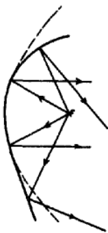
Fig.827.- Shaped mirror for \operatorname{cosec} \theta beam.
