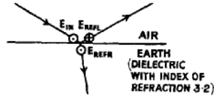
Fig.763.- Horizontally polarised radar waves incident on earth.
